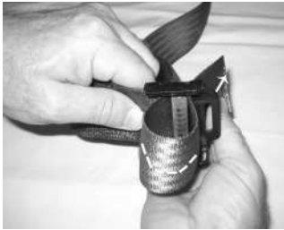
Figure 16 LOOP THE END OVER FLOATING BAR AND BACK THROUGH BUCKLE
