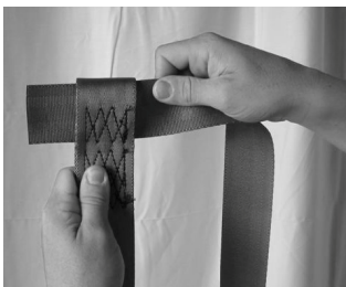
Figure 12 THREAD TREE BELT THROUGH HARNESS LANYARD LOOP
