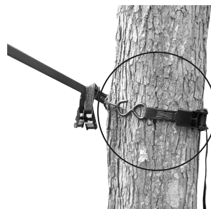
Figure 29 Secure Tree Brace Using Ratchet Strap
