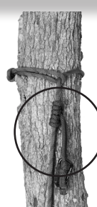
Figure D Prusik Hitch on Loose End Side of Climbing Rope
