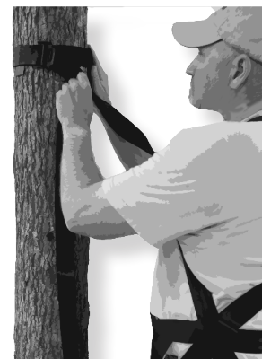
Figure 10 Wrap Tree Belt Around Tree Trunk
