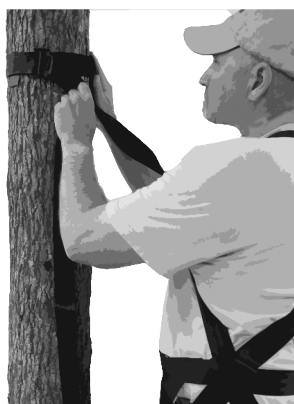
Figure 36 Attach to Full-Body Fall Arrest Tether to Tree Trunk
