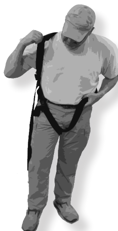
Figure 3 Slip Right Arm Into Right Shoulder Strap
