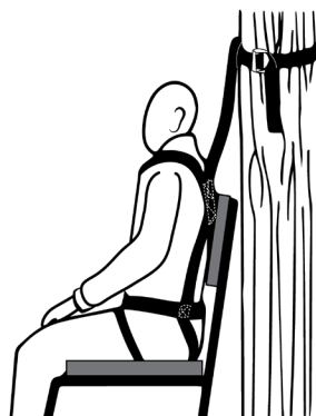
Figure 13 Full-Body Fall Arrest Harness Tether While Seated
