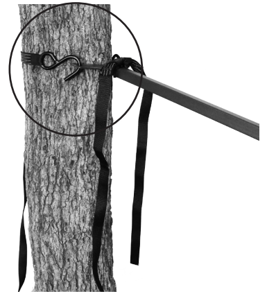
Figure 32 Secure Tree Brace Using Ratchet Strap
