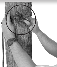
Figure C Slip Knot End Through Loop
