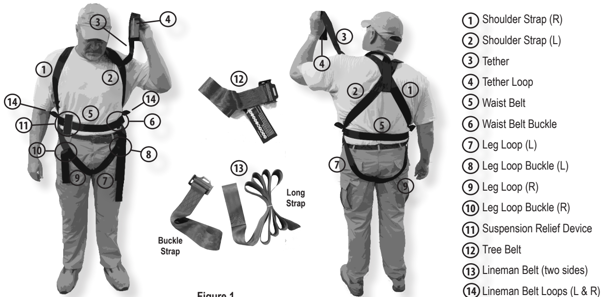
Figure 1 Full-Body Fall Arrest Harness (Front and Rear Views)
