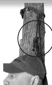
Figure I Position Prusik Hitch as High as Possible
