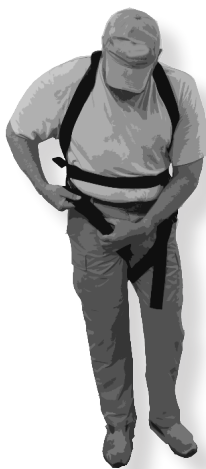
Figure 7 Tighten Leg Loops/Positioned Snugly in Groin Area
