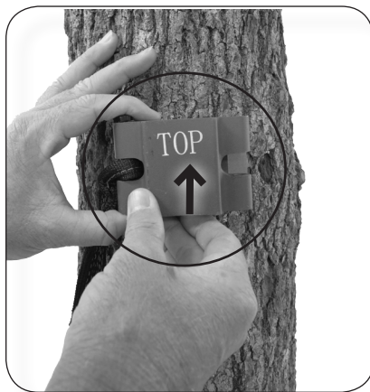
Figure 19 M-102S Receiver Positioned Upward
