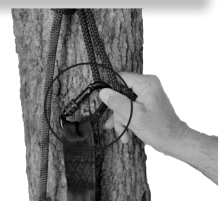
Figure E Carabiner Closed and Locked
