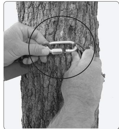
Figure 20 Connect Chain to Quick Link
