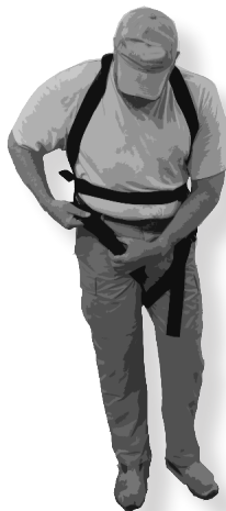
Figure 7 Tighten Leg Loops/Positioned Snugly in Groin Area
