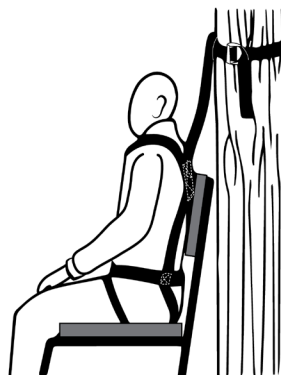
Figure 13 Full-Body Fall Arrest Harness Tether While Seated
