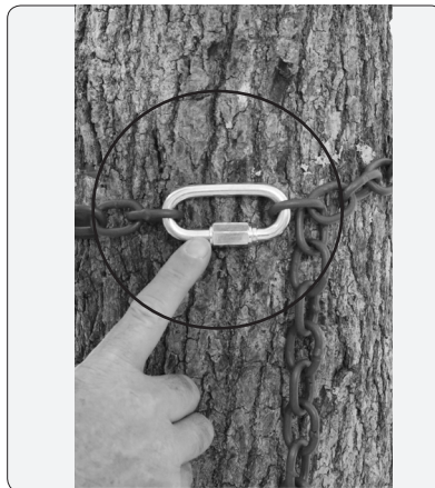
Figure 21 Connect Chain to Quick Link
