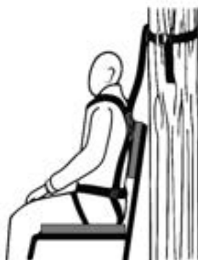
Figure 13 Full-Body Fall Arrest Harness Tether While Seated
