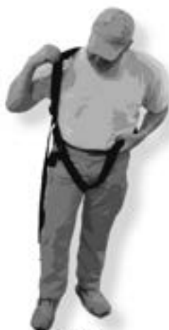
Figure 3 Slip Right Arm Into Right Shoulder Strap
