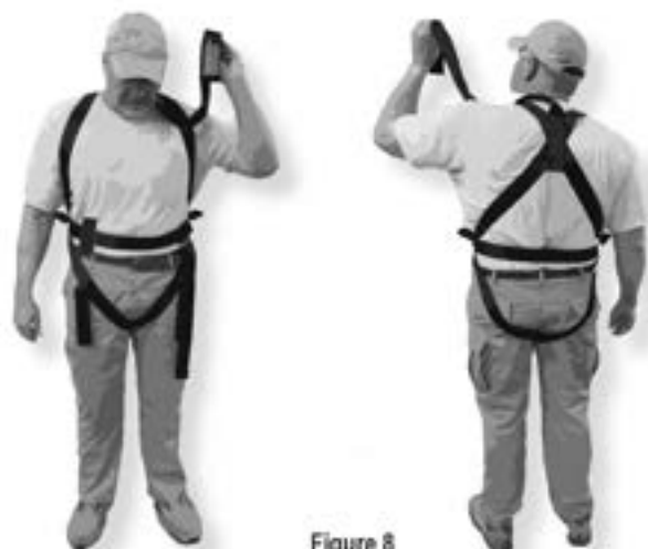
Figure 8 Full-Body Fall Arrest Harness Donned Correctly (Front and Rear Views)
