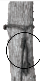
Figure D Prusik Hitch on Loose End Side of Climbing Rope
