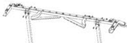
Figure 22 Install Vertical Supports
