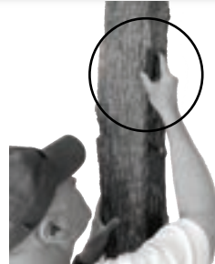
Figure H Slide Prusik Hitch Up Climbing Rope as High as Possible
