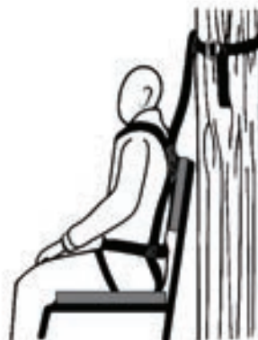
Figure 13 Full-Body Fall Arrest Harness Tether While Seated
