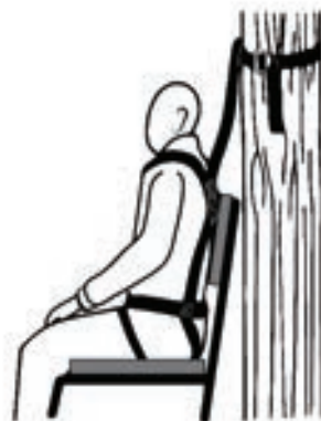
Figure 13 Full-Body Fall Arrest Harness Tether While Seated
