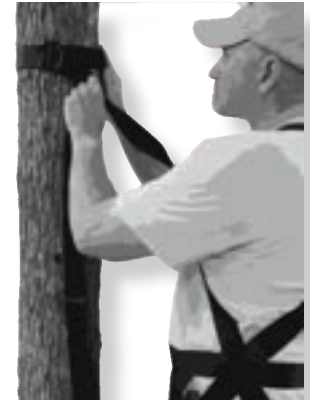
Figure 10 Wrap Tree Belt Around Tree Trunk
