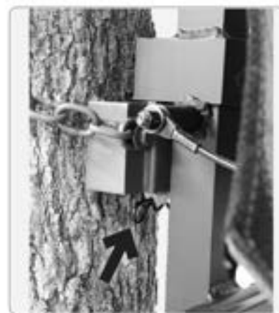
Figure 24 Insert R-Clip Into Receiver Tongue
