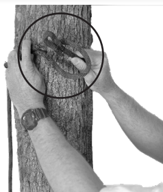
Figure C Slip Knot End Through Loop
