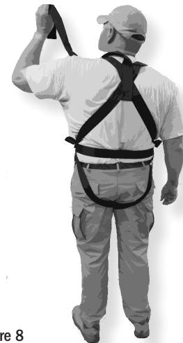
Figure 8 Full-Body Fall Arrest Harness Donned Cor- rectly (Front and Rear Views)
