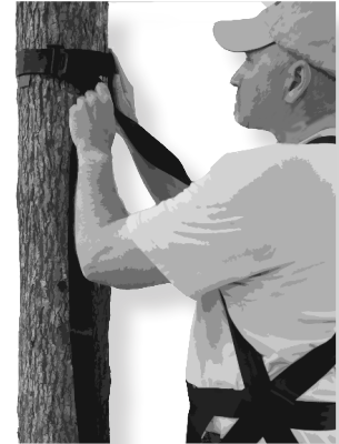
Figure 10 Wrap Tree Belt Around Tree Trunk
